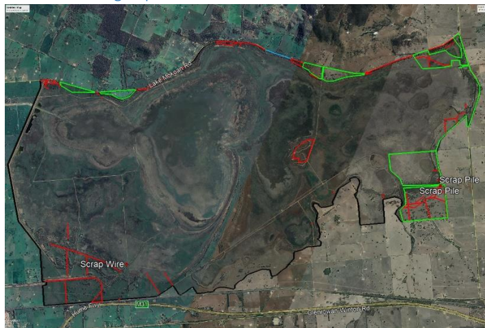
Figure 4. Map of old fencing wire (red lines) removed from Winton Wetlands Reserve throughout 2019
